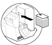
Position the cards with the Smart Card Chip at the top of the card and towards the printer.
